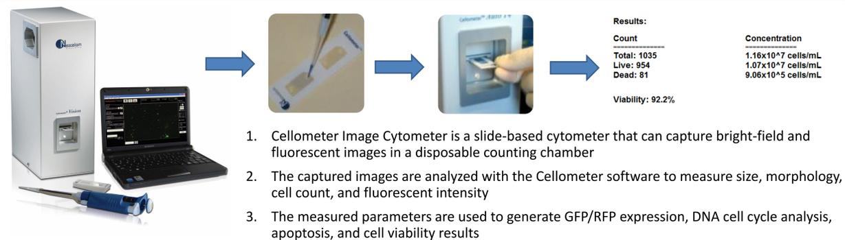
The diagram shows the workflow: 1. Cellometer Image Cytometer is a slide-based cytometer that can capture bright-field and fluorescent images in a disposable counting chamber. 2. The captured images are analyzed with the Cellometer software to measure size, morphology, cell count, and fluorescent intensity. 3. The measured parameters are used to generate GFP/RFP expression, DNA cell cycle analysis, apoptosis, and cell viability results.
