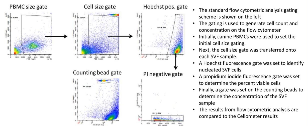
The gating scheme shows: PBMC size gate → Cell size gate → Hoechst pos. gate → Counting bead gate → PI negative gate.
