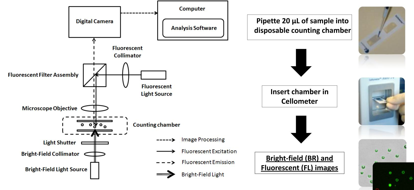
Cellometer image cytometer utilizes an epi-fluorescence setup for fluorescent image analysis
