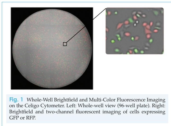
**Fig. 1** Whole-Well Brightfield and Multi-Color Fluorescence Imaging on the Celigo Cytometer. Left: Whole-well view (96-well plate). Right: Brightfield and two-channel fluorescent imaging of cells expressing GFP or RFP.
